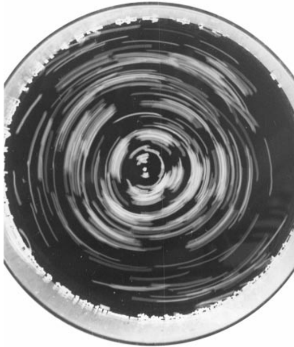
FIGURE 5. An example of streaks from the spin-down experiment at t = 90 s. The exposure time of the camera shutter was calibrated to be 0.961 \text{ s} \pm 0.013 \text{ s} . Although this long shutter time gave overlapping streaks at 90 s it was necessary to assure reasonable accuracy with the shorter streaks at later times.
